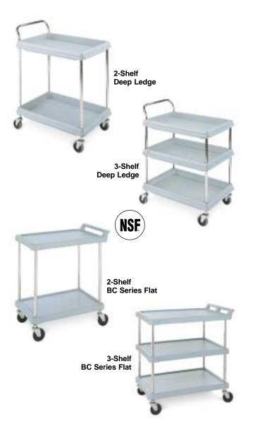
**Specifications:** Utility cart consisting of at least 2 polyethylene, injection-molded shelves containing Microban® antimicrobial product protection, chrome-plated posts or handle. 2-shelf cart may accept an intermediate shelf if necessary. Cart has four 4" (102mm) diameter, resilient rubber swivel stem casters. Cart rated at 150 lbs. (65kg) capacity per shelf, 400 lbs. (180kg) per unit.
